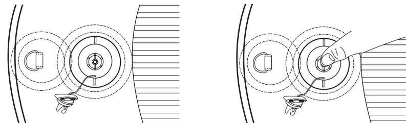
**In the center of the valve is a stem that controls the opening and closing of the valve. To open the valve, press it and turn a quarter turn to lock it in the open position. To shut the valve, turn it a quarter of a turn in the other direction and let the rod come out partially.**
