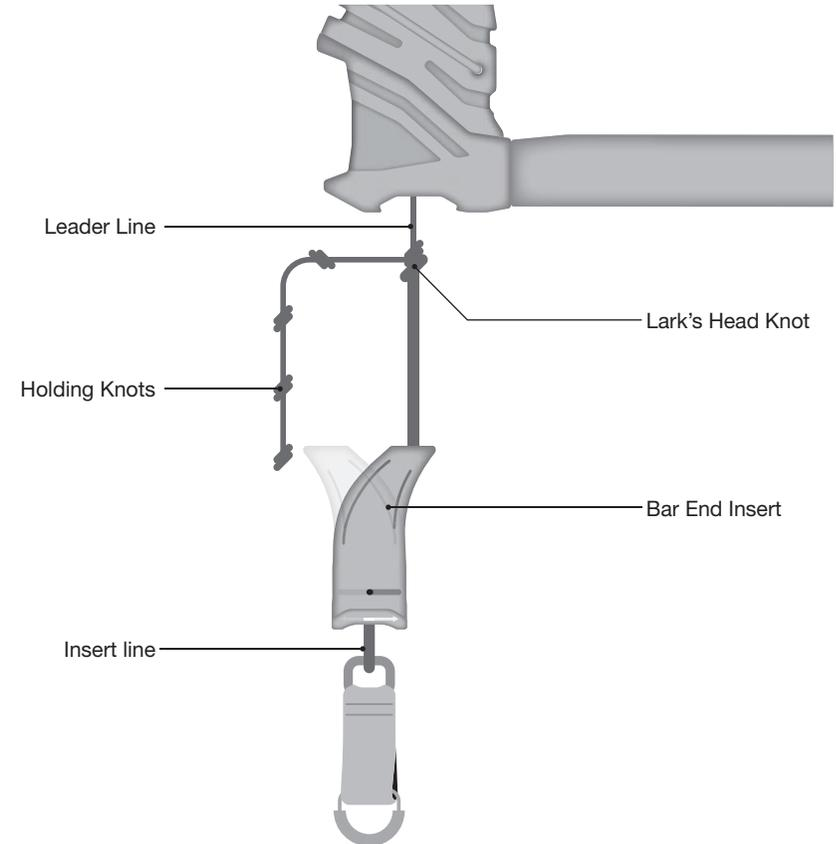
**A succession of holding knots are located at the bottom of the Leader Lines to adjust the length of the backlines. To do so, follow the procedure:**
