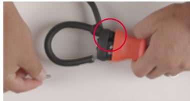
2. Unscrew the chicken loop retaining screw.
