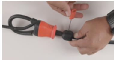
2. Unscrew the QR retaining screw at the roto head.
