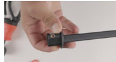
3. Remove the stainless steel cylinder holding the line.
