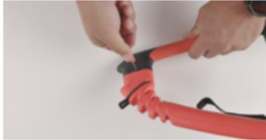
1. Unscrew the floater screw using the tool provided in the bar bag.
